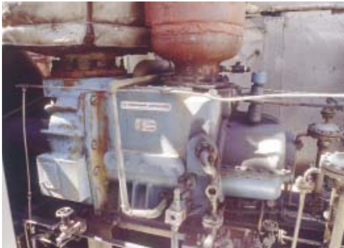
Electric Driven Screw Compressor w/ Kaydon Face Bushing Seals ■
